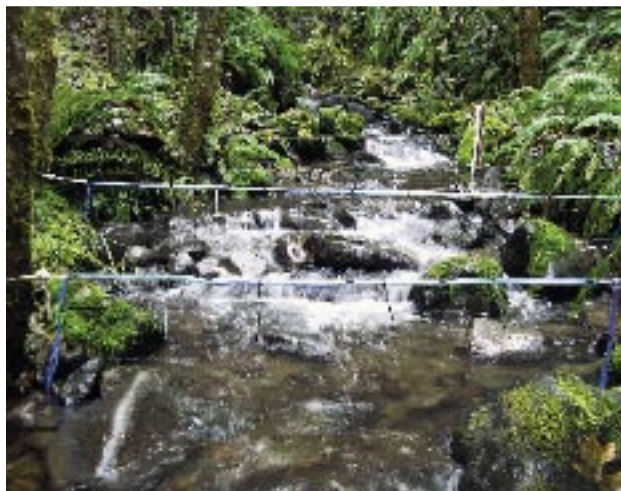
Sophisticated gate readers span the creek at numerous locations. As the fish with implanted PIT (Passive Integrated Transponder) tags pass under them, the gate readers can identify the exact fish, enabling scientists to track their movement throughout the watershed and their response to disturbance. This new technology was not available to researchers during the earlier studies that inform current forest practices laws.
